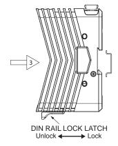
the cradle until flush with the rail and push the DIN rail lock latch to the latched (in) position.
