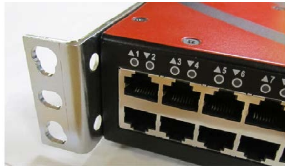
Figure 1-3. Brackets Front Flush or Setback Mounted
