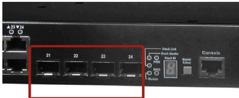
Figure 1-2. Gigabit / SFP Ports 21-24
