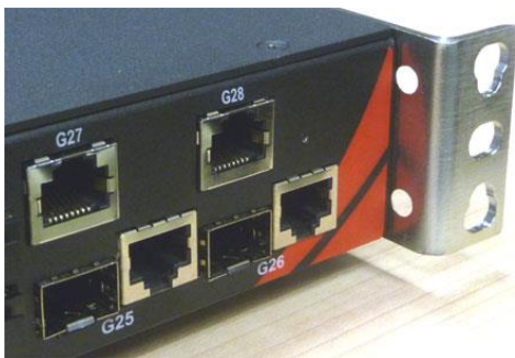
In the image above, the brackets are mounted so the front of the switch is setback 1/2 inch.
