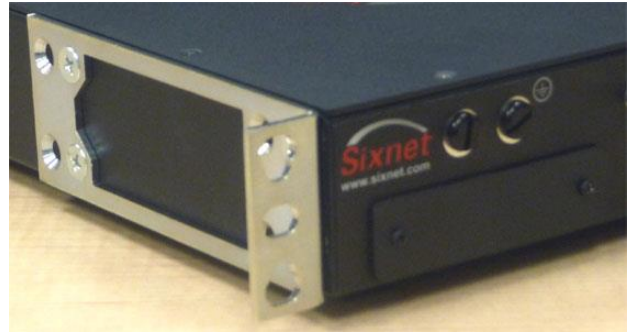
In the image above, the brackets are mounted flush with the back of the switch.
