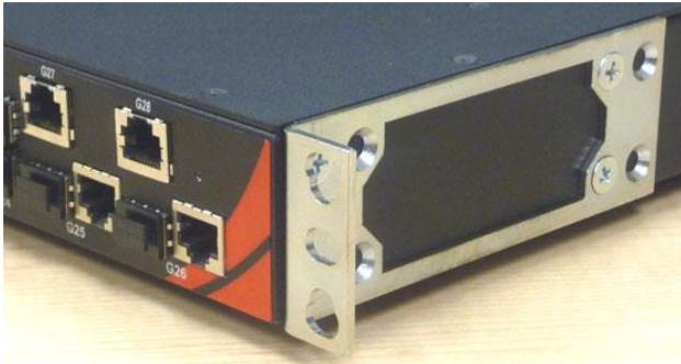
In the image above, the brackets are mounted flush with the front of the switch.
