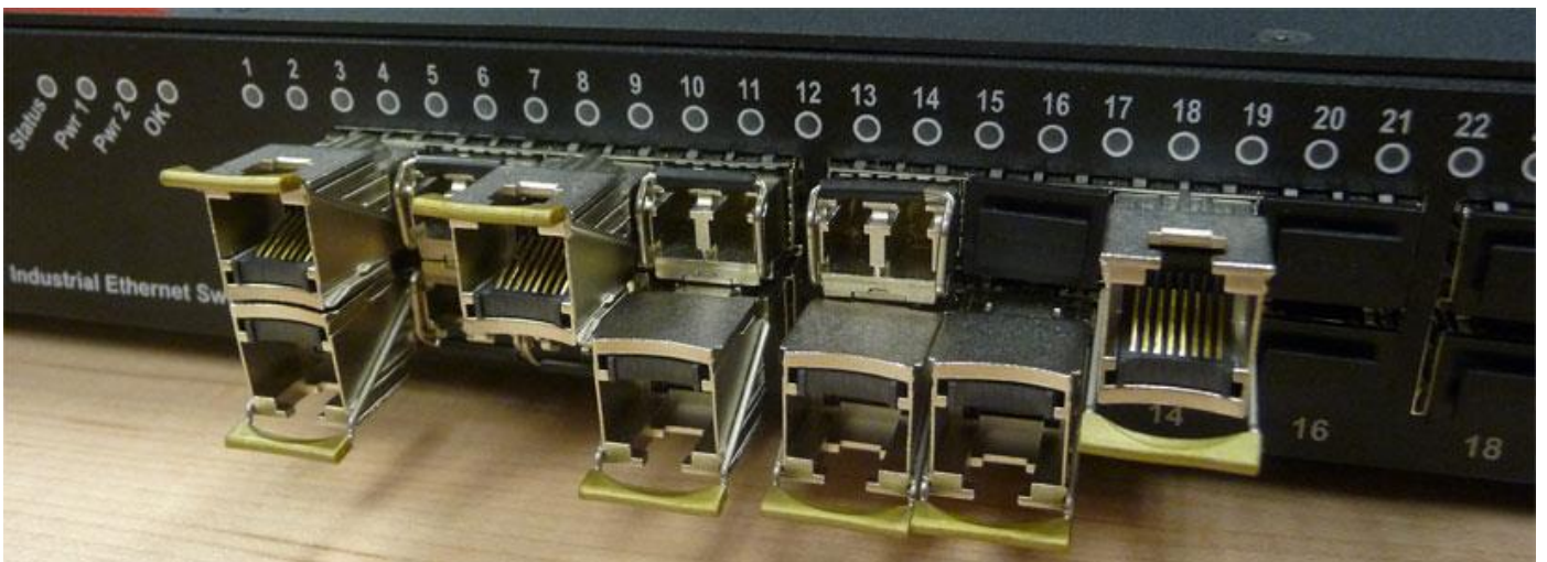
Mix and Match SFP Transceivers as Desired (use supplied plugs to cap unused ports)
