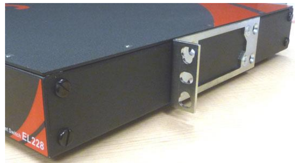
In the image above, the brackets are mounted in the middle of the switch to accommodate a centrally located rail.
