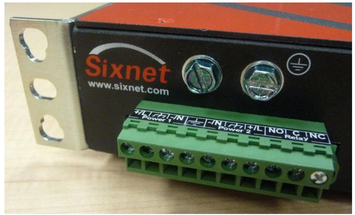
Power Plug Installed
