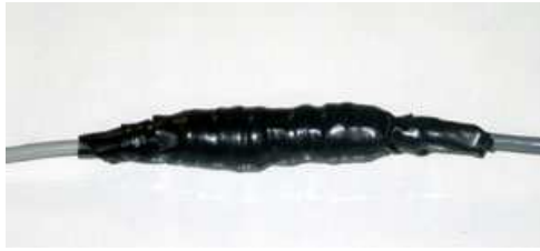
Figure 25. Example of a connector pair sealed with self-amalgamating tape
