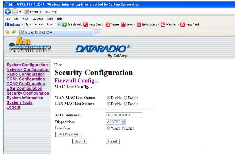
Image 6-34: Firewall Configuration, MAC List Config. Submenu
