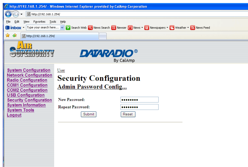
Image 6-25: Security Config., Admin Password Config. Submenu
