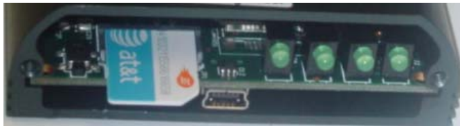
Figure 3-2: Insert SIM in to the modem
