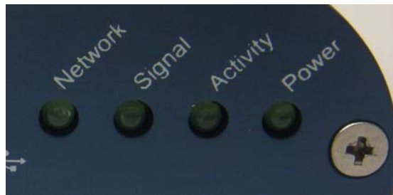
Figure 4-5: Raven XE Indicator lights
