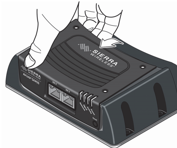
Figure 2-13: Tilting the cover (Dual Ethernet X-Card installed)
