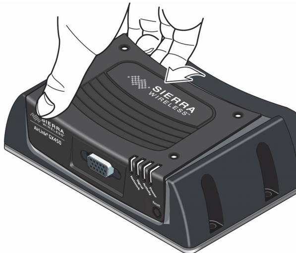
Figure 2-8: Tilting the cover (I/O X-Card installed)
