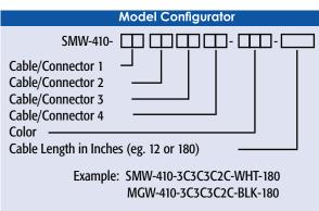
Specify "SMWG" or "MGWG" instead of "SMW" or "MGW" for GPS/Glonass combination antenna.
