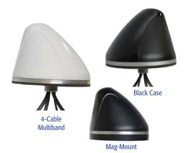
The SMW-410 Series Antennas features 4 elements in one antenna radome. The unique feature of this model is that it offers two identical high gain elements covering 2.4 GHz & 4.9-6.0 GHz. Of the remaining two elements in the SMW-410, one is used for GPS at 1575 MHz and the other covers 2.1-2.5 GHz & 4.4-6.0 GHz. All three elements offer an impressive 5 dBi gain.
