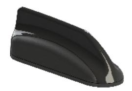
Mobile Mark's MXF702 Series Multiband Diversity/MIMO antenna contains seven separate antenna elements, all in one compact antenna housing: two broadband LTE/Cellular antennas, four dual-band WiFi antennas, and one GPS antenna. The MXF702 covers Cellular LTE frequencies from 694-3700 MHz.
