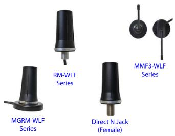
The RM-WLF wideband Series are 3 dBi gain broadband antennas. A ground plane is recommended for best performance. These antennas will operate over the entire 694-894 MHz spectrum, along with 1.7-2.7 GHz high frequency spectrum.
