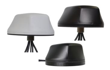
Mobile Mark's LTM507 Series Multiband Diversity/MIMO antenna contains five separate antennas, all in one compact antenna housing: two broadband LTE/Cellular antennas, one dual-band WiFi antenna, one Iridium antenna and one GPS antenna. The LTM507 differs from the LTM501 in that it covers the Iridium frequencies from 1616-1626.5 MHz.
